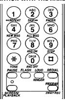
olf the SCREEN/PLAYBACK indicator flashes when you press SCREEN/PLAYBACK, the answering system is off. To turn it on, press "8".
