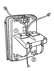
Connect the telephone line cord. Mount the unit, then slide down.
