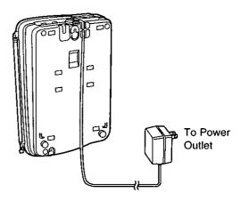
Tuck the telephone line cord inside the wall mounting adaptor.
